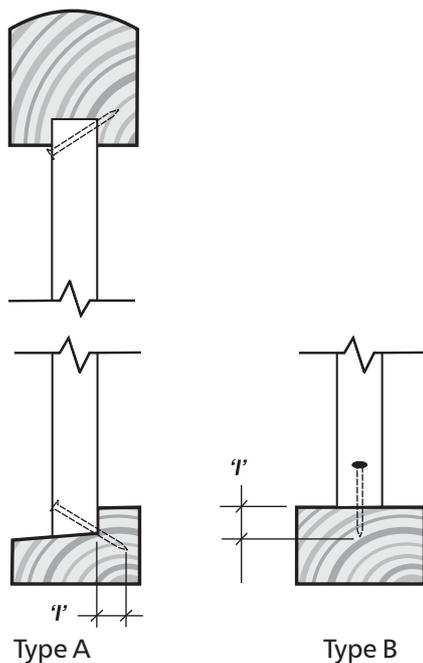
**Figure 5. Balusters/Infill**
